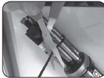
Figure 8 - Carefully cut away excess length from the secured zip-tie
