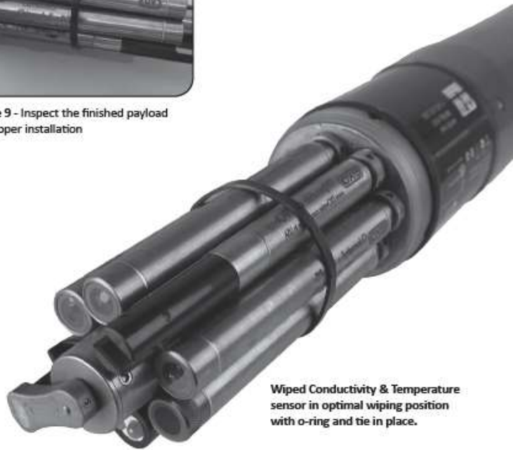
Figure 10 - Finally, to ensure that the zip tie is out of the way, place the sensor guard back on the sonde.
