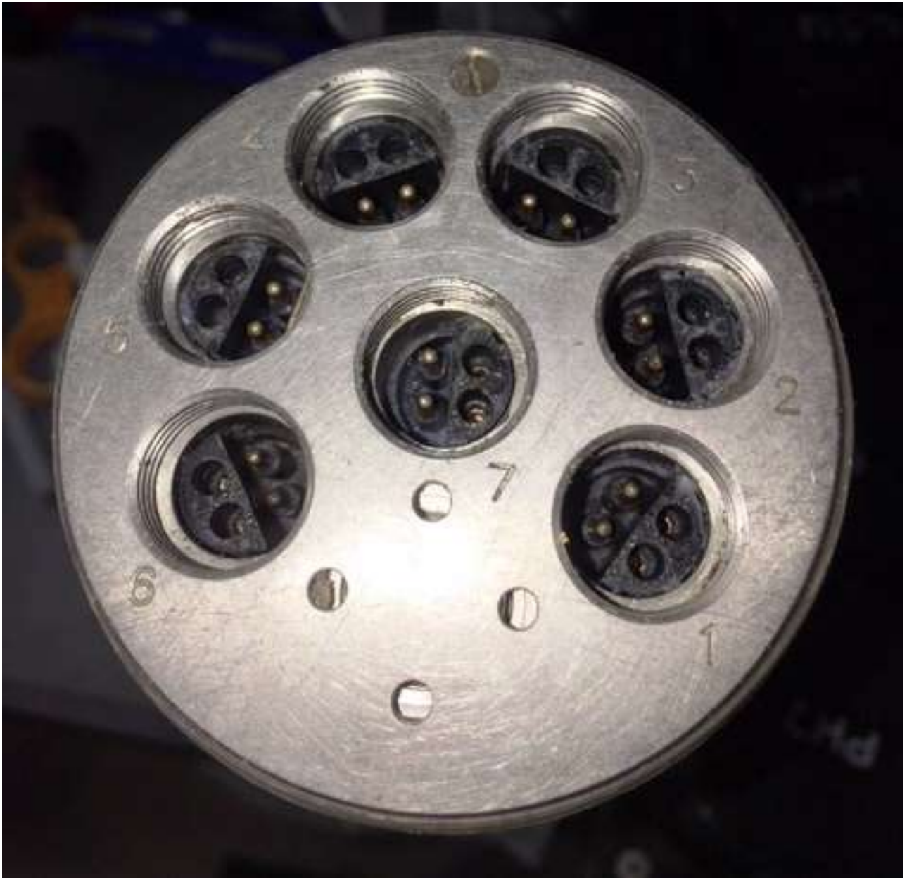
EXO Bulkhead with Typical Contaminates
