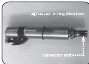
Figure 1 - Roll on the new o-ring starting at the connector end
