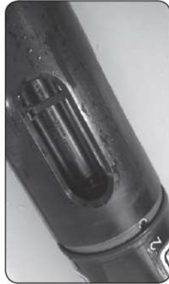
Figure 10 - Finally, to ensure that the zip tie is out of the way, place the sensor guard back on the sonde.
